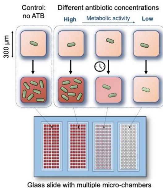
Figure 1: Conceptual sketch of the microfluidic system for antibiotic susceptibility testing (AST). The platform consists of hundreds of growth chambers (300 x 300 x 75 μm), each pre-filled with oxygen sensing nanoprobes and different concentrations of the studied antibiotics (ATBs) embedded in the agarose gel. The metabolic activity of bacteria after exposure to antibiotics is determined based on oxygen consumption.
