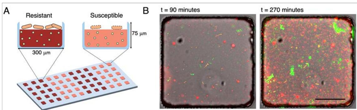
**Figure 1.** A: Scheme of the system. B: A growth chamber containing different *E. coli* strains in co-culture. One strain is resistant to ampicillin (green-sfGFP), while the other is susceptible (orange-mKate2). The chamber also contains oxygen-sensing particles (red); bacteria are consuming oxygen and the luminescence signal of the particles increases.
